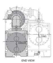
Fig. 32 — 19XR Insulation Area
